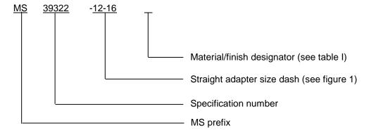
PIN example: MS393221-12-16 indicates an adapter nipple, -12 of the PIN indicates a 3/4 inch (19.05 mm) swivel nut with 1.063 - 12 UN-28 threads: -16 of the PIN indicates weld socket to accommodate 1-inch tubing, steel with cadmium plate.
