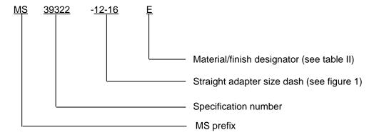
PIN example: MS393221-12-16E indicates an adapter nipple, -12 of the PIN indicates a 3/4 inch (19.05 mm) swivel nut with 1.063 - 12 UN-28 threads: -16 of the PIN indicates weld socket to accommodate 1 inch tubing, steel with NAVAIR TCP.
