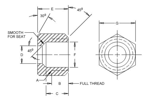
FIGURE 1. Nuts, tube coupling – safety sleeve compression type.
