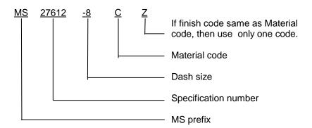
Guidance on use of alternative parts with less hazardous or non-hazardous materials. This specification provides an alternate material, corrosion resistant steel, and Zinc finish via the PIN. Users should select the PIN with the least hazardous material that meets the form, fit, and function requirements of their application.
