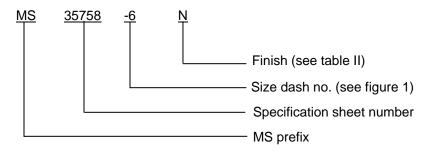
Example of a PIN: M35758-6R, is a steel, 1 ounce, manual feed grease cup that is zinc plated in accordance with ASTM-B633; type VI, Fe/Zn 5.
