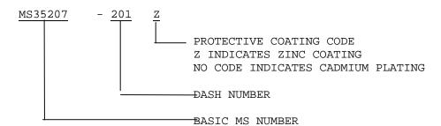
MS35207-201Z INDICATES - SCREW, MACHINE-PAN HEAD, CROSS-RECESSED, CARBON STEEL, ZINC COATED, .086-56, UNC-2A, .125 LENGTH.
