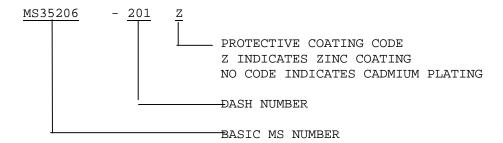
MS35206-201Z INDICATES - SCREW, MACHINE-PAN HEAD, CROSS-RECESSED, CARBON STEEL, ZINC COATED, .086-56, UNC-2A, .125 LENGTH.
