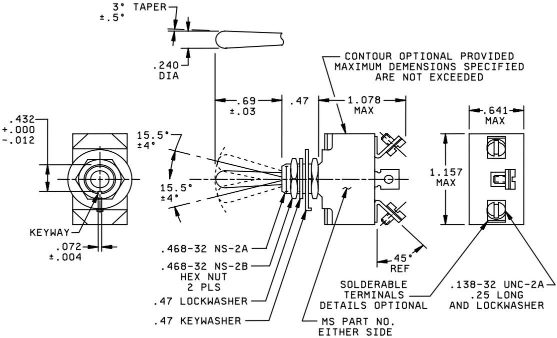
FIGURE 1 Dimensions and configurations
