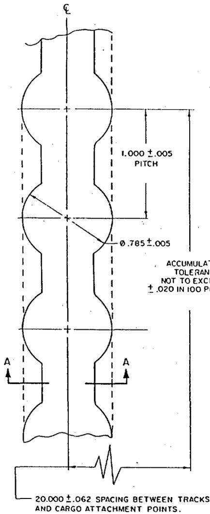
ACCUMULATED TOLERANCE NOT TO EXCEED ± .020 IN 100 PITCHES
