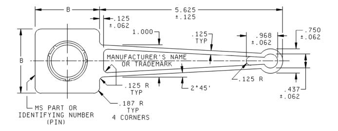
FIGURE 1. Tool, dimensions and configurations.
