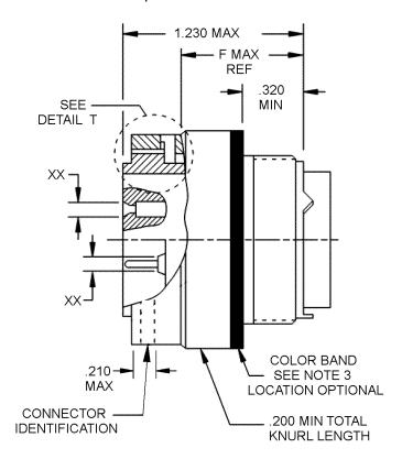
NOTE: For "XX", note 5 and table I for contact cavities requiring reduced dimensions.
