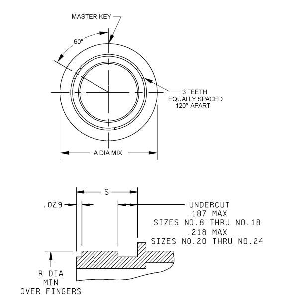
DETAIL T (COUPLING RING REMOVED FOR CLARITY)
