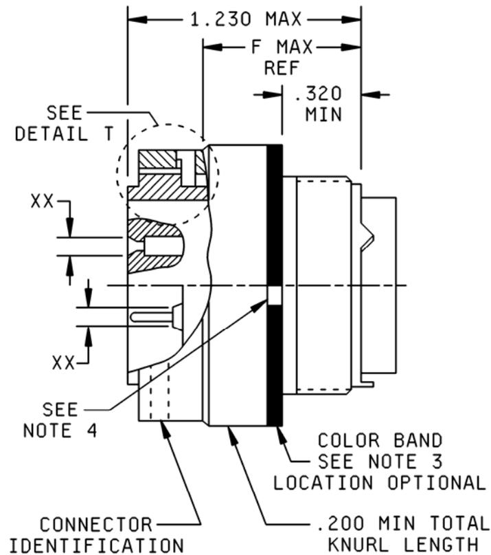
NOTE: For "XX", see note 4 and table I for contact cavities requiring reduced dimensions.
