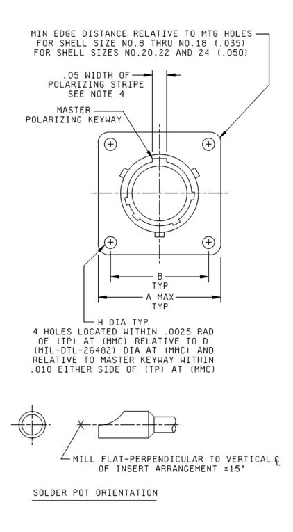
FIGURE 1. Receptacle, class H, dimensions and configurations - Continued.
