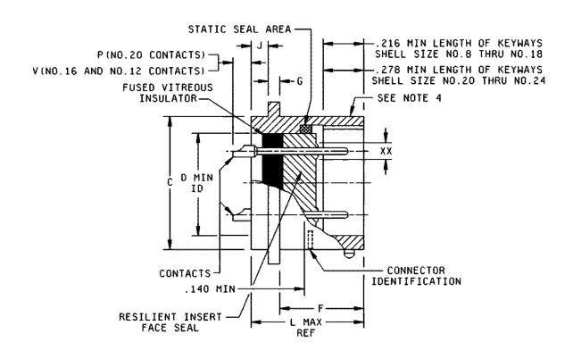
NOTE: For "XX", see note 5 and table I for contact cavities requiring reduced dimensions.
