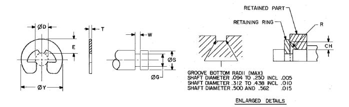
FIGURE 1. Ring, Retaining.
