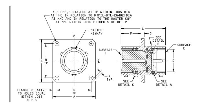
FIGURE 1. Receptacle, class E, dimensions and configurations.
