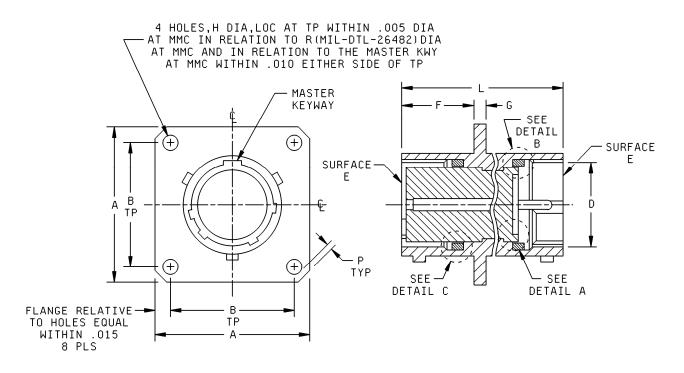
FIGURE 1. Receptacle, class E, dimensions and configurations.
