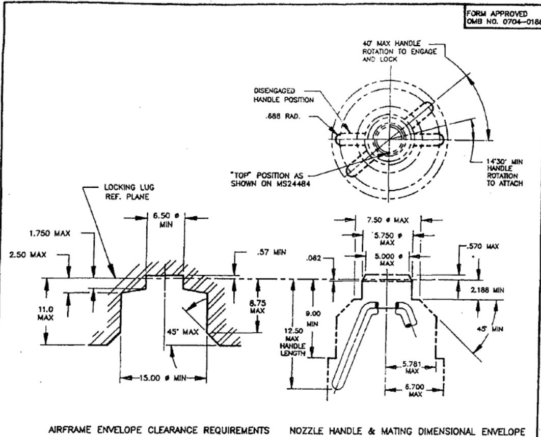
AIRFRAME ENVELOPE CLEARANCE REQUIREMENTS NOZZLE HANDLE & MATING DIMENSIONAL ENVELOPE
