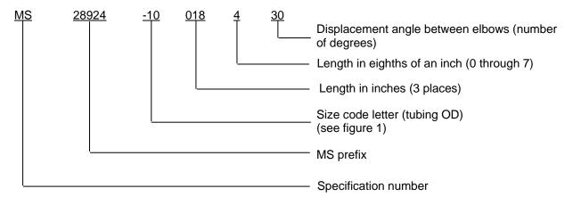
Example of a PIN: MS28924-10018430, MS28924 hose assembly, .625 inch (5/8 inch) passageway diameter, 18.5 inches long, 30° ±2° angular displacement.
