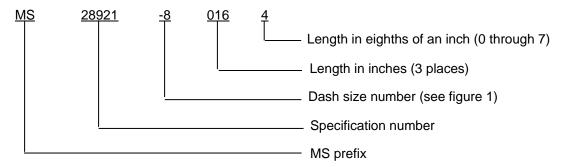
Example of a PIN: MS28921H0164, MS28921 hose assembly, .500 inch (1/2 inch) passageway diameter, 16.5 inches long.
