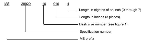
Example of a PIN: MS28920-100164. MS28920 hose assembly, .625 inch (5/8 inch) passageway diameter, 16.5 inches long.
