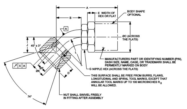
FIGURE 1. Fitting end, 45° elbow, flared tube dimensions and configuration.
