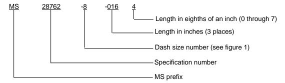
Example of a PIN: MS28762-8-0164, MS28762 hose assembly, .500 inch passageway diameter, 16.5 inches long.
