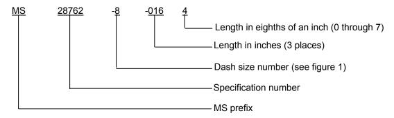
Example of a PIN: MS28762-8-0164, MS28762 hose assembly, .500 inch passageway diameter, 16.5 inches long.
