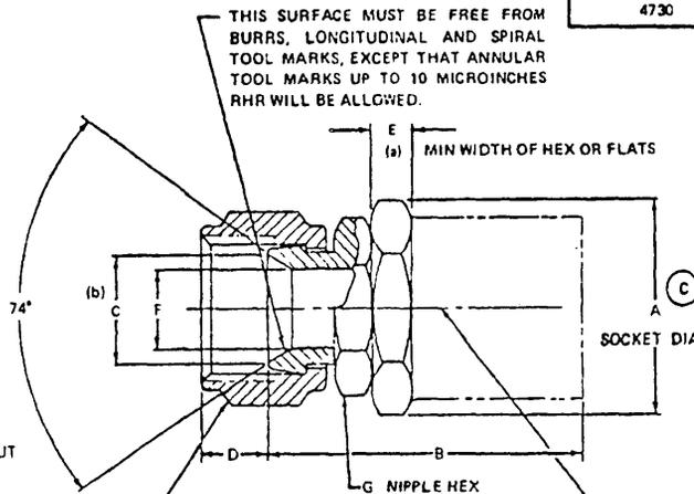
THIS SURFACE MUST BE FREE FROM BURRS, LONGITUDINAL AND SPIRAL TOOL MARKS, EXCEPT THAT ANNULAR TOOL MARKS UP TO 10 MICROINCHES RHR WILL BE ALLOWED.
