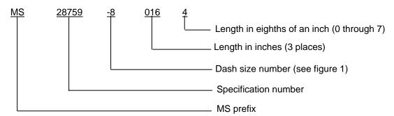
Example of a PIN: MS28759-80164. MS28759 hose assembly, .500 inch (1/2 inch) passageway diameter, length 16.500 inches.
