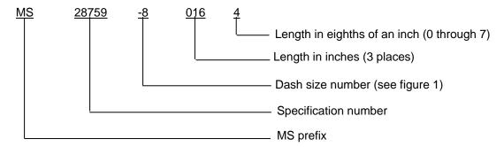
Example of a PIN: MS28759-80164. MS28759 hose assembly, .500 inch (1/2 inch) passageway diameter, length 16.500 inches.
