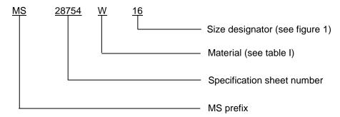
Example of PIN: MS28754W16 indicates a swivel with 45° flange, aluminum, 1-inch hose or tubing size.
