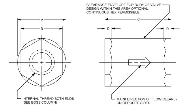
FIGURE 1. Valve, check, low pressure, internal threads.
