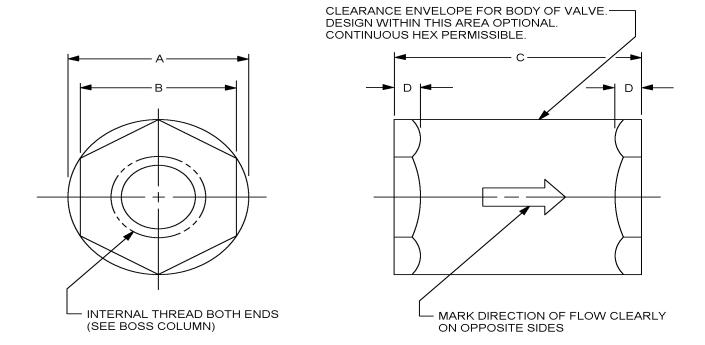
FIGURE 1. Valve, check, low pressure, internal threads.
