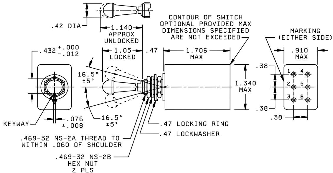
FIGURE1. Dimensions and configuration
