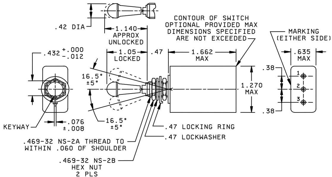
FIGURE1. Dimensions and configuration
