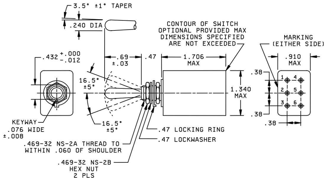
FIGURE1. Dimensions and configuration
