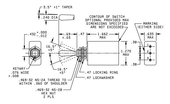
FIGURE1. Dimensions and configuration
