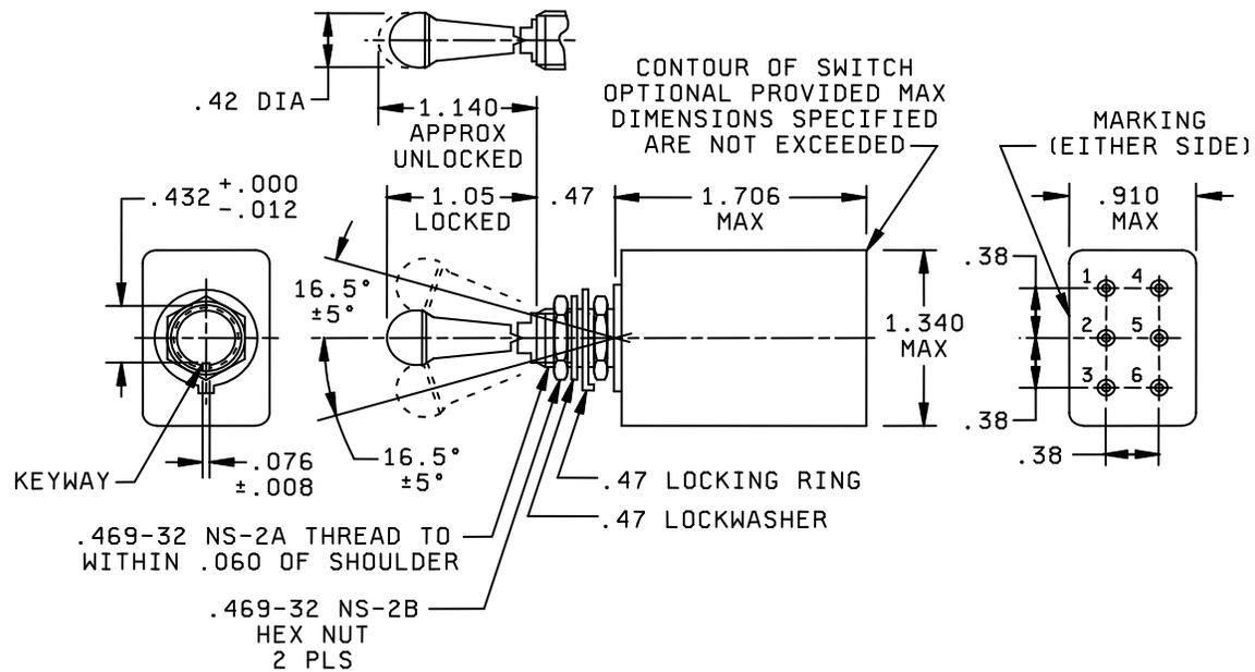
FIGURE1. Dimensions and configuration
