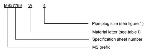
PIN example: MS27769W4 indicates a pipe plug, aluminum alloy 7075-T73, 3/8 -18 ANPT.
