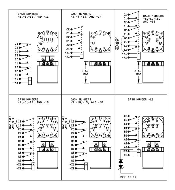
NOTE: When semiconductors are required, JANTX or equivalent screened semiconductors shall be used. Relays using suppression devices shall continue to operate if the suppression circuit is in a failure mode. Diodes shall have a peak inverse voltage of 600 V dc min.
