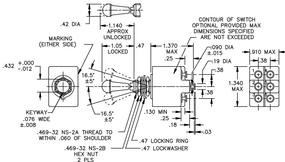
FIGURE 1. Dimensions and configuration
