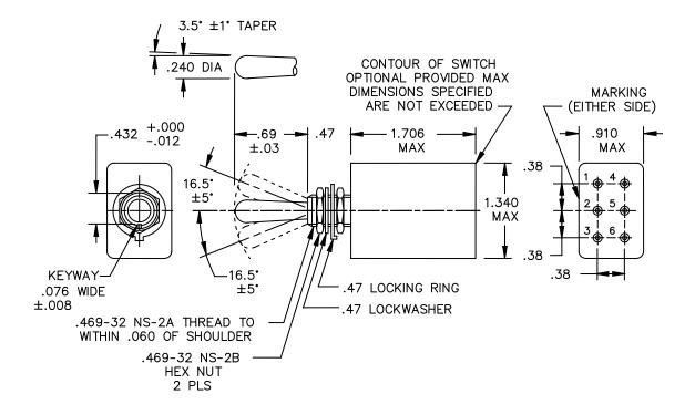
FIGURE1. <u>Dimensions and configuration</u>
