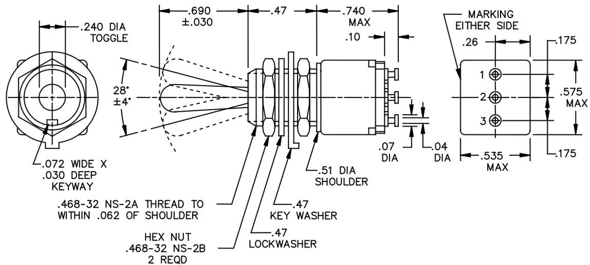
FIGURE 1. Dimensions and configurations
