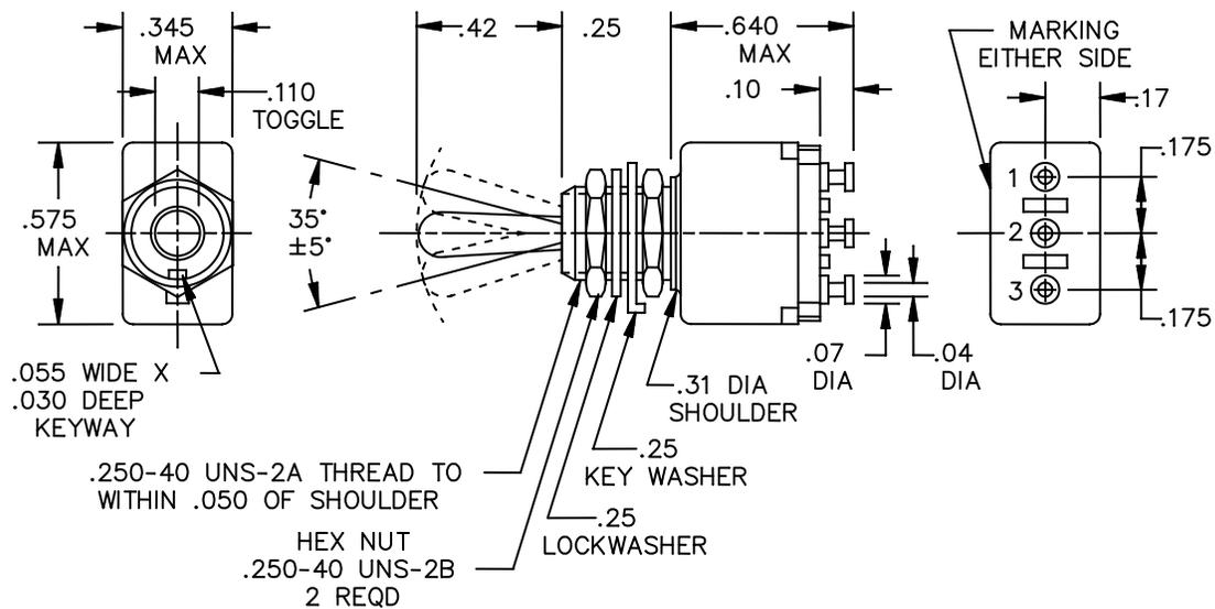
FIGURE 1. Dimensions and configurations
