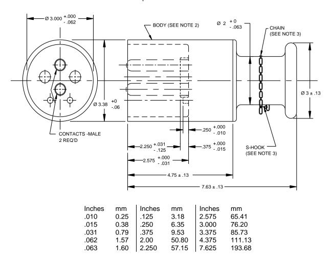
FIGURE 1. Contact, ramp power, 412/240 volts, large female.
