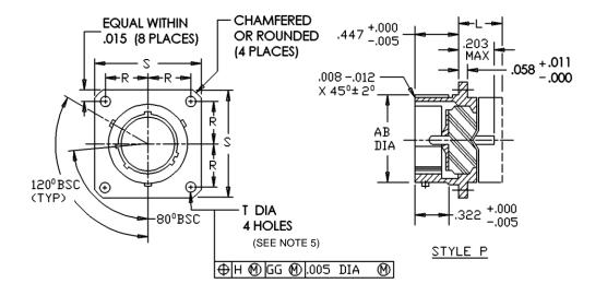
FIGURE 1. Receptacle, classes E, T, and P.
