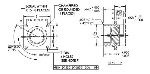
FIGURE 1. Receptacle, classes E, T, P and V.
