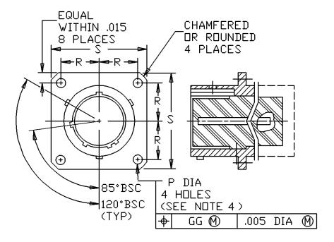
FIGURE 1. Receptacle, classes E, T and P.
