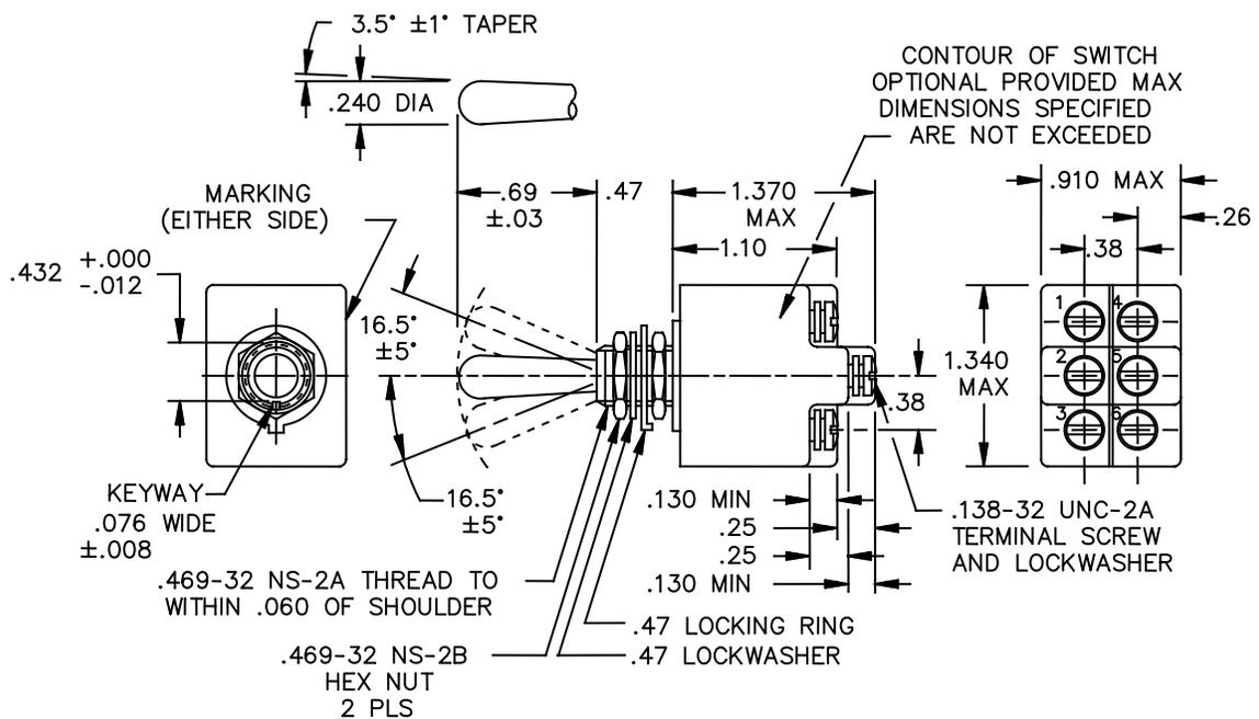
FIGURE1. Dimensions and configuration
