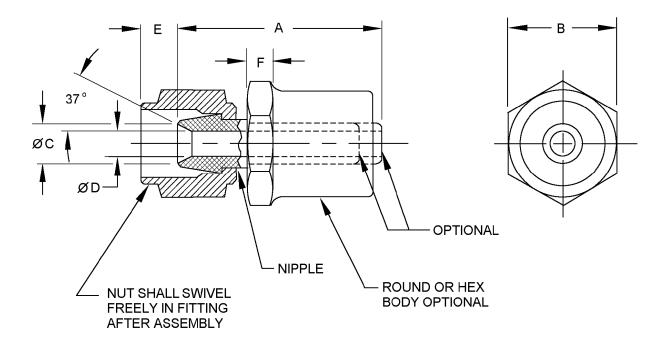
FIGURE 1. Adapter dimensions and configuration.
