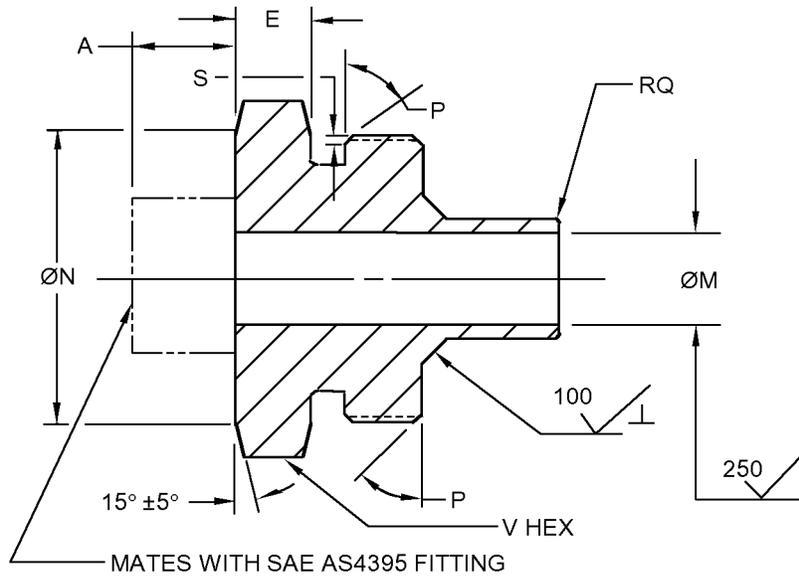
FIGURE 1. Nipple illustration - Continued.TABLE I. Nipple requirements.
