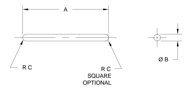
FIGURE 1. Wire retainer
