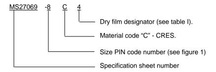
Example: MS27069-8C4 indicates: .500 inch tube OD, socket to hose coupling fitting, corrosion resistant steel, with dry film class designator 4.
